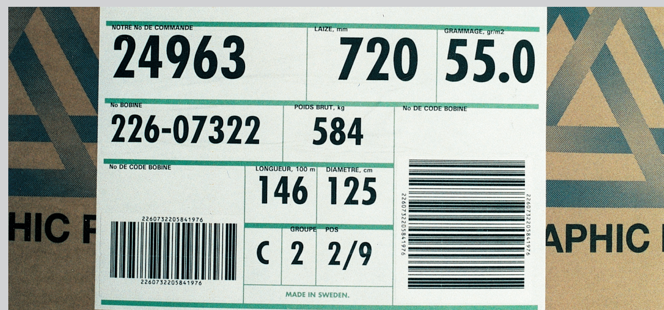
This information provides essential data on paper use and allows rolls to be traced in the event of paper problems.
